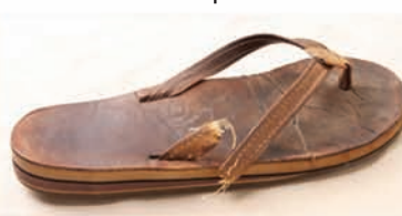
Torn side straps
